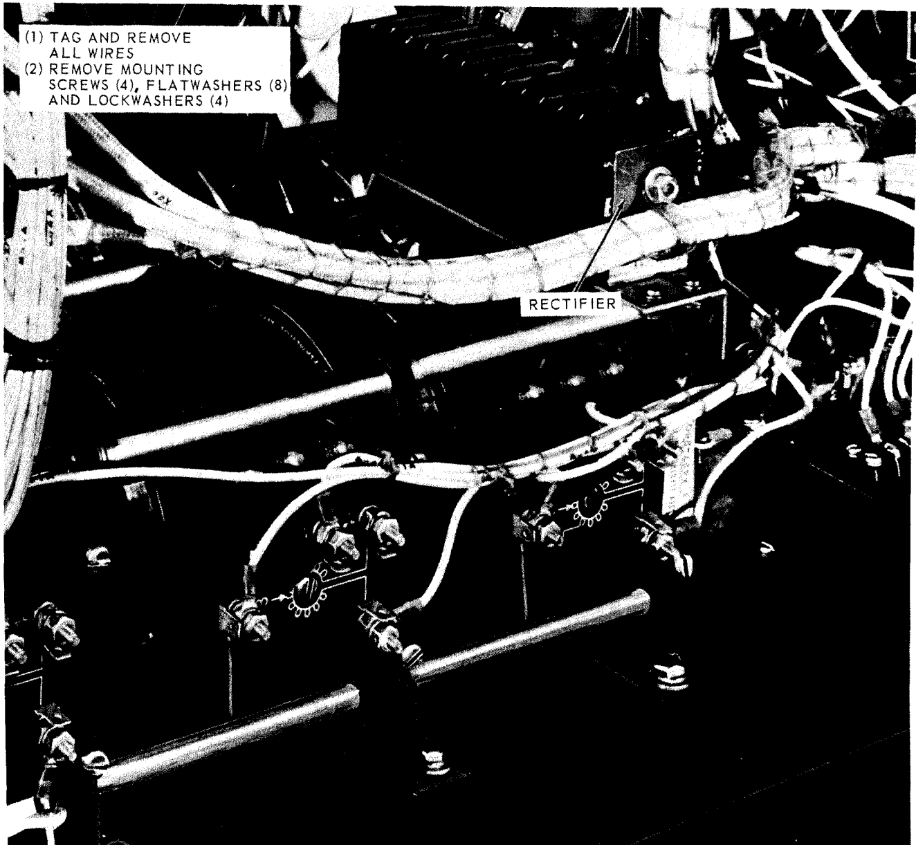
Figure 5-1. Rectifier removal and installation. Table 5-1. Troubleshooting (Cont'd).
